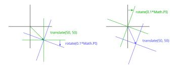
But if we *first* rotate by 20 degrees and *then* translate by (50, 50), the translation will happen in the rotated coordinate system and thus produce a different orientation. The order in which transformations are applied matters.
