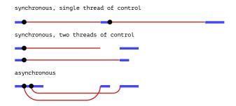
Another way to describe the difference is that waiting for actions to finish is *implicit* in the synchronous model, while it is *explicit*—under our control—in the asynchronous one.
