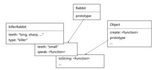
Overriding properties that exist in a prototype can be a useful thing to do. As the rabbit teeth example shows, overriding can be used to express exceptional properties in instances of a more generic class of objects while letting the nonexceptional objects take a standard value from their prototype.
